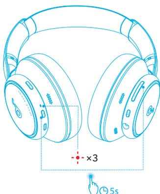
You might need to reset your headphones if you experience connectivity or function issues. Delete the pairing history from your Bluetooth device first. Press the power and volume up buttons simultaneously for 5 seconds until the LED flashes red three times.
