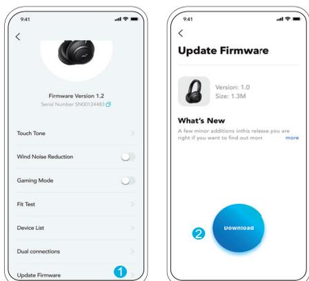
You will be informed once the new version of firmware is detected when you connect the headphones with the app. Ensure the headphones are powered on and connected to a device until the firmware update is complete. During the update, avoid any usage and ensure stable access to the internet.
