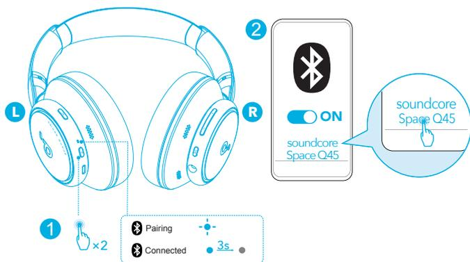
The headphones can connect with two devices at the same time. When already connected to one device, press the power button twice to pair with another device.
