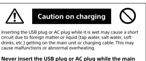
Inserting the USB plug or AC plug while it is wet may cause a short circuit due to foreign matter or liquid (tap water, salt water, soft drinks, etc.) getting on the main unit or charging cable. This may cause malfunctions or abnormal overheating.
