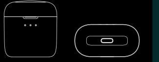
Note - The LED lights located on the charging case indicate the battery status of the case.
